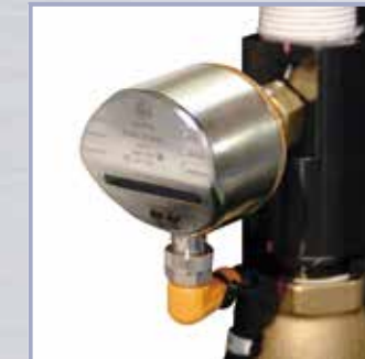
Coolant flow switch
